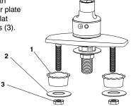
Install spout nut (1) onto the spout.
